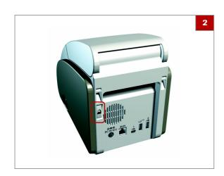
**2** Press the lid button at the back of the instrument and open the lid.
