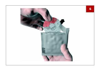
4 Remove the test disc from the pouch holding the hinge cover of the disc with thumb and forefinger or thumb and middle finger.
