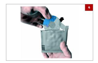
4 Remove the test disc from the pouch holding the hinge cover of the disc with thumb and forefinger or thumb and middle finger.
